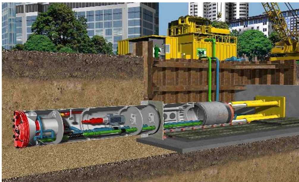
Plate 3.10: Indicative micro-tunnelling schematic
